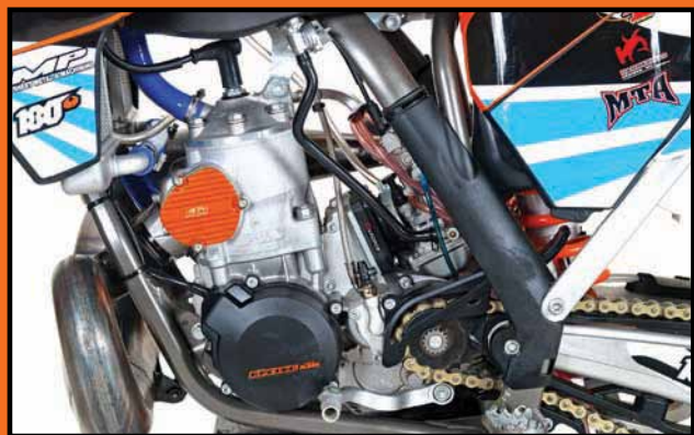
Intelajet provided a means for fuel-flow adjustability via their Dial-A-Jet. Dial-A-Jet is like a power jet, but it has air bleed, so instead of feeding raw fuel like a power jet, the device meters the air and mixes it with the fuel in a chamber, delivering a pre-atomized fuel mixture into the center of the carb throat. www.thunderproducts.com
