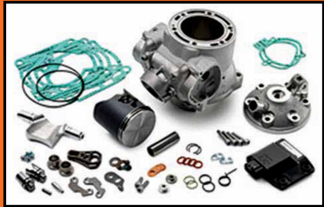
Here's the 300 conversion kit from KTM's Power Parts division.
